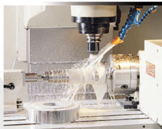
High pressure coolant (P:3.5 kg/cm 2 , Q:100 l/min)
