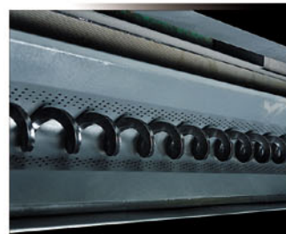
Automatic chip removal (Screw type chip conveyor)
