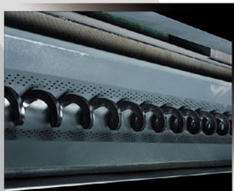
Automatic Chip Removal (Screw Type Chip Conveyor)
