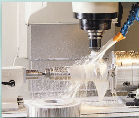
High Pressure Coolant (P:3.5 kg/cm 2 , Q:100 ℓ/min)
